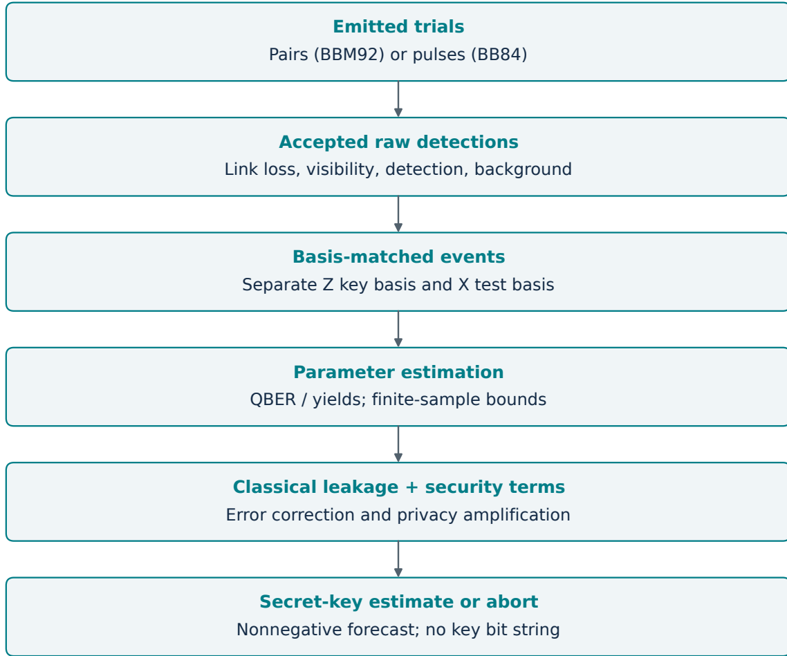
Figure 12: The count pipeline distinguishes emitted trials, accepted detections, basis-matched data, parameter-estimation bounds and the final secret-key estimate. BBM92 emitted trials are pairs; BB84 emitted trials are pulses. A rate or fraction is meaningful only with its denominator and integration duration. All displayed outputs remain forecasts.
